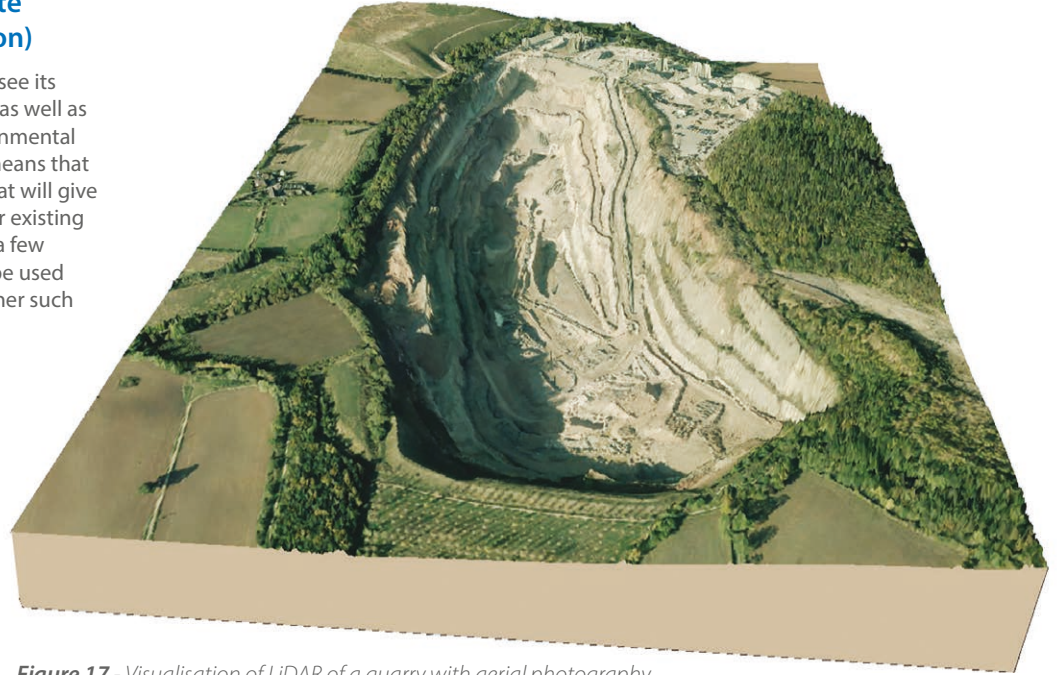
Figure 17 - Visualisation of LiDAR of a quarry with aerial photography
